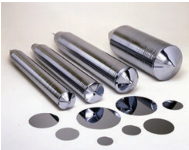
Figure 3.11: Silicon ingots and polished wafers.
